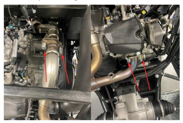
Install the 2 powdercoated brackets we supply, as the picture shows. The bolts that are being used are the M6 x 20 yellow plated, 2 of them don't need any nut as there are threads in the frame, and the other 2 will use the flange nuts supplied (yellow plated).
