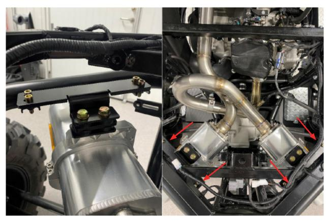
Install the header pipes as the picture shows (don't forget the stainless clamp on the pipe with a sleeve and slots). The center bracket on the pipes uses one M6 x 20 allen bolt with a flange nut on the backside. Don't tighten this down until everything is bolted up. Use the M8 x 70 hexagon bolts for the spring loaded coupling and washers. Use the factory flange nuts on the cylinder flange/pipe.
