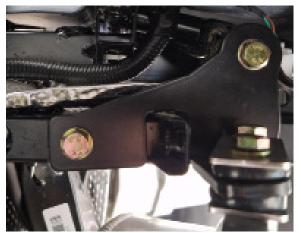
**Important note!** Looking at the APX from the back of the vehicle, the bracket you use on the LEFT APX can has a small 'cut out' in the center of it.
