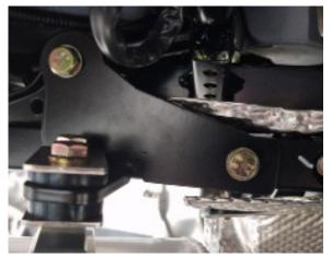
**Important note!** Looking at the APX from the back of the vehicle, the bracket you use on the RIGHT APX is solid. There is no 'cut out'.
