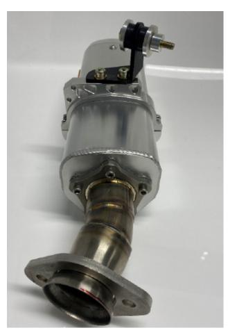
Install the bolt washers and aluminum spacers as the picture shows.
