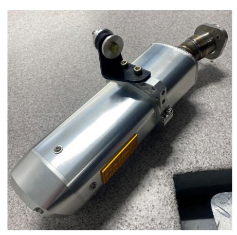
Step 5 - Install the stainless inlet pipe, use the exhaust gasket with 5 holes in between the muffler and pip flange. Use the M6 x 20 stainless allen bolts and the M6 lock washers tighten them down evenly. See the picture below on how to align the inlet pipe.
