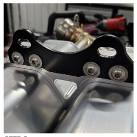
Use 4x M8x20 Screws to attach the Black Exhaust Bracket to the bottom of the Stainless Steel Clamp as seen in the above image.
