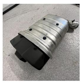
**STEP 1.** Remove the factory muffler.
