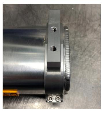
The second clamp needs to be installed 89 mm (3.5") from the end of the muffler where the endcap sits. This can be adjusted later on, but it's better if you do it properly now.
