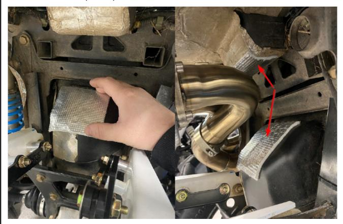
Slide the exhaust on the header pipe and let the exhaust hang until you installed the rear bumper back. Make sure to slide the stainless clamp on before as it is not possible to do afterward. Use a string/strap if needed to support the exhaust during installation, so you don't bend the header pipe as there is a lot of weight.
