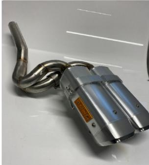
Install the inlet pipe as the picture shows and slide the stainless clamp on the pipe. Use the supplied exhaust gaskets between the muffler and stainless flanges. Tighten down the clamp as much as you can.
