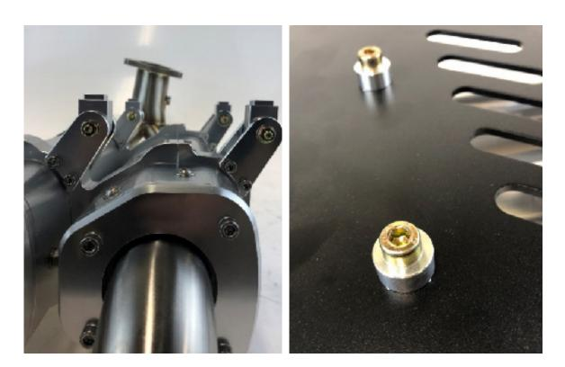
*Step 4 -* Install the stainless inlet pipe on the lower muffler and the 5 hole gasket included with the hardware. Don't forget to use the gaskets. See picture below.
