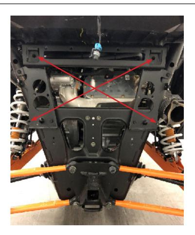
**Step 6** – Install the u-pipe as the pictures below shows, use the m6x20 ss allen bolts with lock washers and don't forget to use the gasket included. We recommend a thin layer of the supplied anti seize on the clamps bolt so you can tighten it harder no specific torq are recommended on the bolt tighten it as hard as you can by hand and re-tighten it after the first ride.
