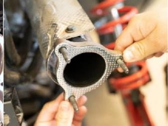
**Step 6** – Install the u-pipe as the pictures below shows. Use the m6x20 ss allen bolts with lock washers and don't forget to use the gasket included. We recommend a thin layer of the supplied anti seize on the clamps bolt so you can tighten it harder. No specific torq are recommended on the bolt tighten it as hard as you can by hand and re-tighten it after the first ride.
