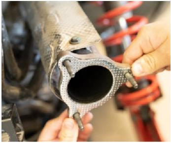
**Step 8** – Install the muffler package on the frame and line it up with the header flange to make sure everything sits as it should. Then tighten everything down.
