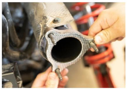
**Step 5** – See the picture below on how to install the inlet pipe. All exhausts comes with the m12x1.25 lambda bung hole plugged . If you need to use it just remove the plug from the hole and install the sensor. Use the supplied gaskets see the picture below .
