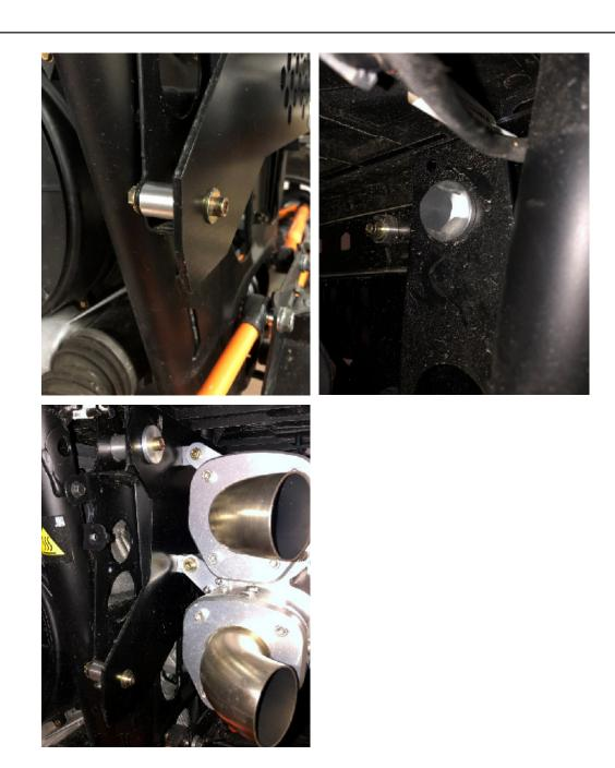
*Step 7 -* Start the engine let the vehicle idle for 15 min, then turn it off and let it cool down then re-tighten all the bolts.
