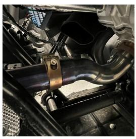
**STEP 13.**Use the second Exhaust Clamp to secure the mid pipe to the header pipe.
