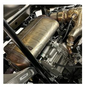
**STEP 2.** After the two bolts have been removed, you should now be able to slide the stock exhaust out.
