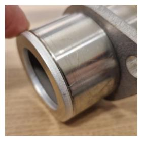
To help with the fitment of the header pipe, you can use the provided aluminum ring inbetween the gasket and the cylinder.
