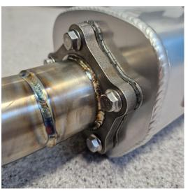
**STEP 2.**Place the 1x Exhaust Gasket between the Pipe and the APX can.
